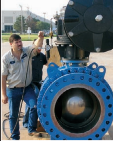
Cycle testing a Series VT3 24" FP Class 600 with pneumatic spring return actuator for ESD service at ViNtrol's Oklahoma City manufacturing facility.
