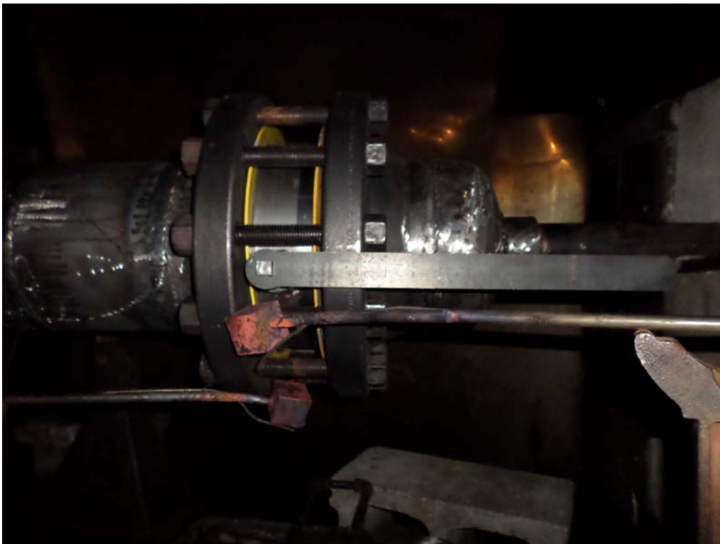
Test Valve Setup Prior to Burn
