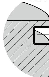
**WARNING:** AREA IN BOLD IS A CRITICAL AREA. DAMAGE TO THE AREA MAY REDUCE OR ELIMINATE THE SEALING FUNCTION OF THE PLUG.
