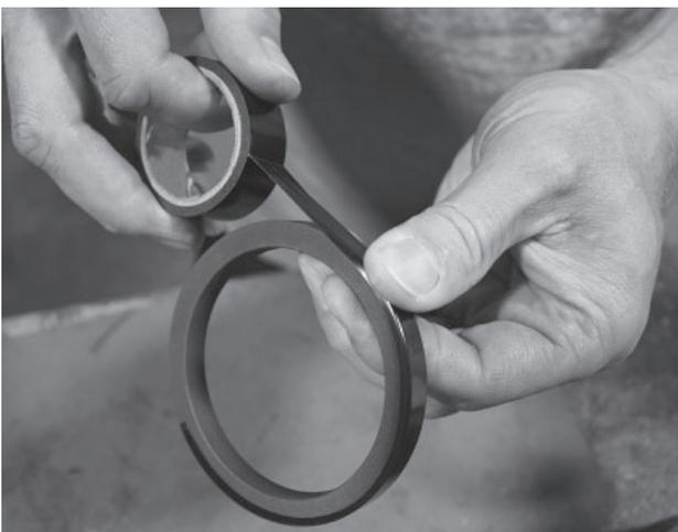
**Figure 23** Model 351 Piston Ring Vise Break Method (Step 1)
