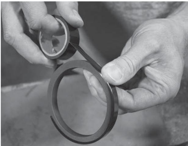
**Figure 21** Model 361 Piston Ring Vise Break Method (Step 1)
