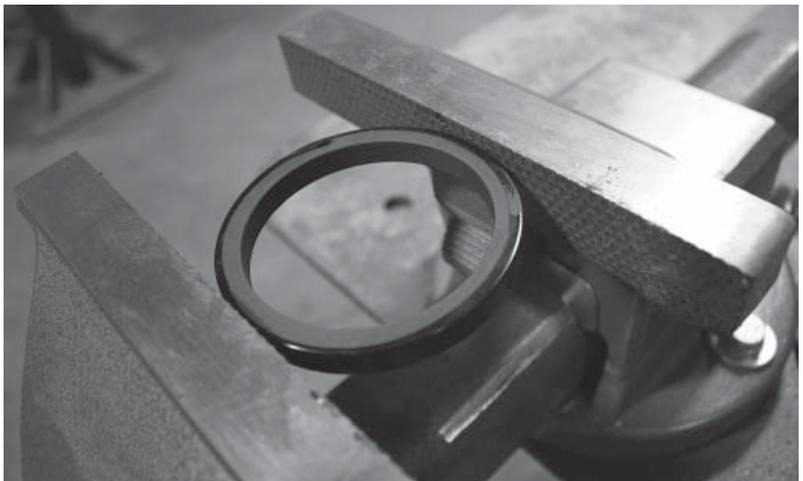
**Figure 22** Model 361 Piston Ring Vise Break Method (Step 2)
