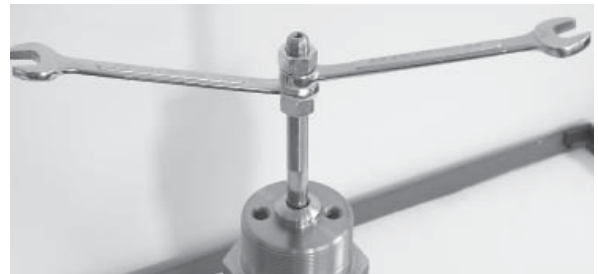
Figure 6 Handle Construction for Lapping
