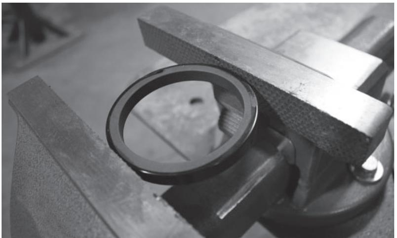
**Figure 21** Piston Ring Assembly for Model 391 Valves (Step 2)
