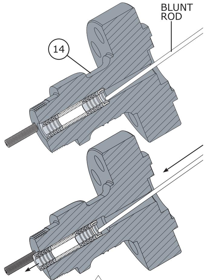
**Figure 13** Packing Parts Removal (Step 1)
