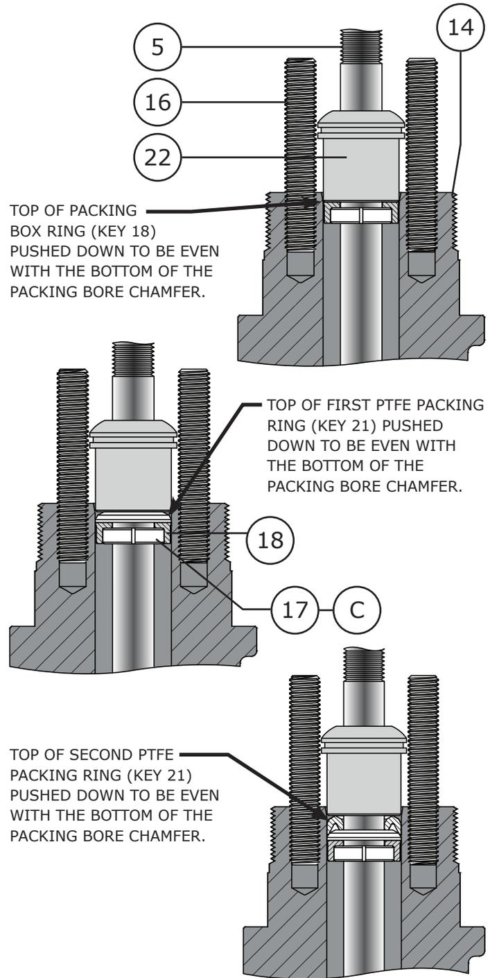
**Figure 25** Proper Packing Ring Installation
