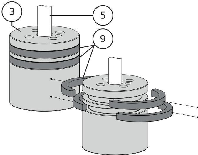
**Figure 11** Model 391 Piston Ring Removal
