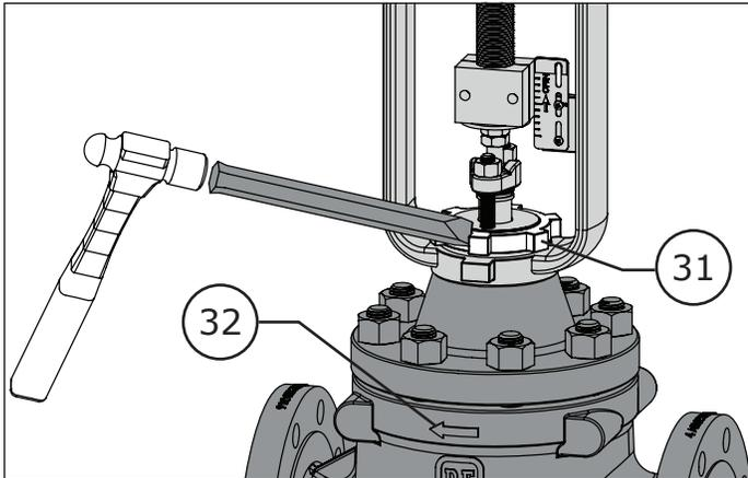
**Figure 4** Yoke Nut being loosened with a Chisel
