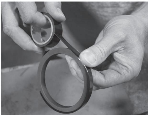
**Figure 20** Piston Ring Assembly for Model 391 Valves (Step 1)
