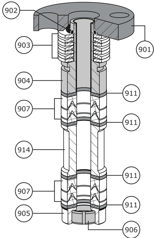
**Figure 30** Live Loaded Packing Example
