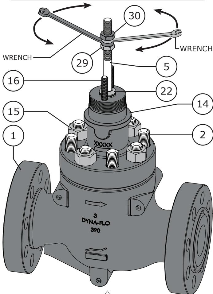
**Figure 16** Lapping Procedure Setup (Steps 9 - 10)
