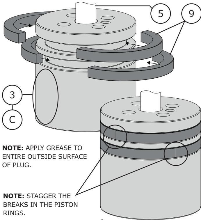
**NOTE:** APPLY GREASE TO ENTIRE OUTSIDE SURFACE OF PLUG.
