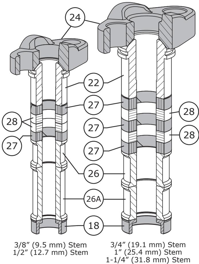
**Figure 29** Single Graphite Packing Arrangement
