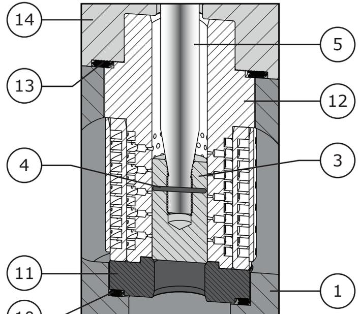
**Figure 36** *Anti-Cavitation Trim Detail*
