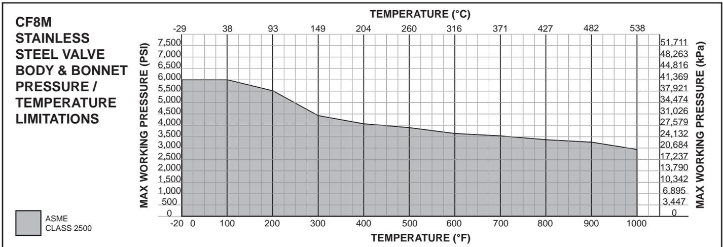
**Maximum Inlet Temperature and Pressures** - Valves consistent with ASME Class rating as per ASME B16.34, unless limited by either material, pressure or temperature limitations.
