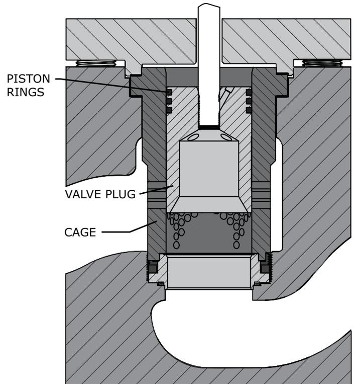
**Figure 7** Model 381 Plug and Cage Design
