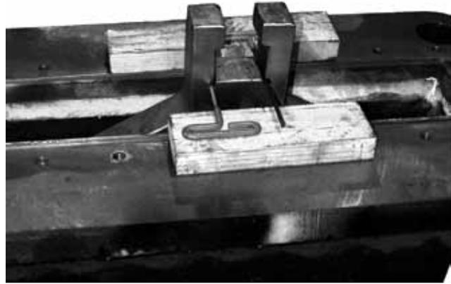
**5.6.8** Slide the stem T-bar out of the T-bar slot in the gate neck. This will disengage the top works assembly from the gate allowing its removal. Remove the bonnet O-ring.
