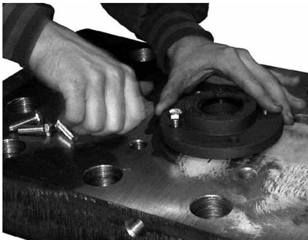
**5.6.19** Approaching from the bottom of the bonnet, insert the new stem through the stem packing. Be careful not to damage the stem packing. Let the stem protrude from the bottom of the bonnet approximately the same amount as the old stem. Tighten the capscrews holding the bolted stem packing retainer to bonnet.
