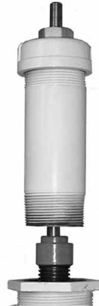
**5.3.6** Remove bonnet nuts. Studs may also be removed, if desired, to allow more work clearance.
