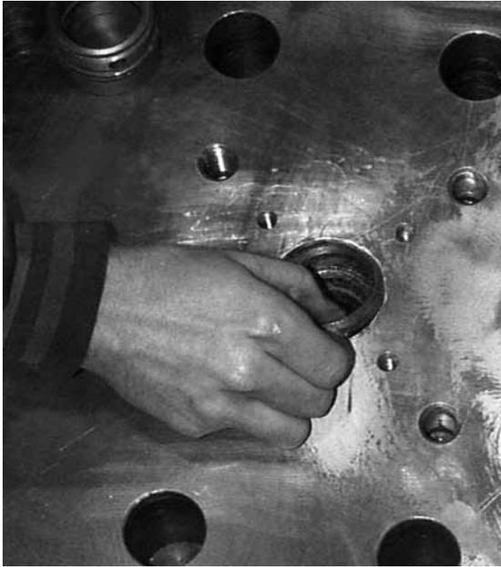
**NOTE: Be careful not to damage the stem seal area of the stem when sliding the bonnet over the stem.**
