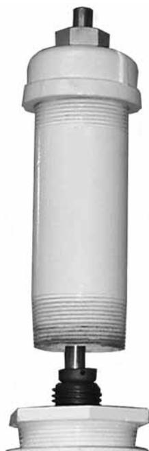
**5.5.6** Remove bonnet nuts. Studs may also be removed if desired to allow additional work clearance.
