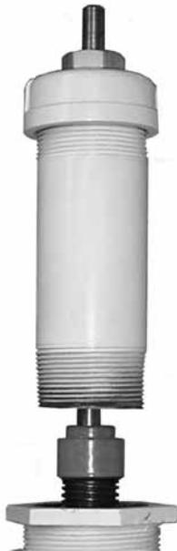
5.1.6 Remove bonnet nuts. Studs may also be removed if desired to allow more work clearance.
