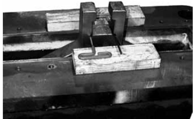
5.8.8 Slide the stem T-bar out of the T-bar slot in the gate neck. This will disengage the top works assembly from the gate allowing its removal. Remove the bonnet O-ring.
