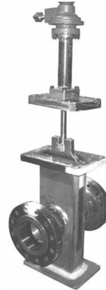
**5.5.7** Using proper equipment and lifting procedures, lift the entire top works assembly, bonnet, and gate high enough to clear the T-bar slot in the gate. Insert customer supplied drift pins in the holes provided in the bottom of the gate T-bar slot.
