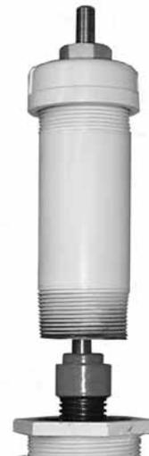
5.2.6 Remove bonnet nuts. Studs may also be removed, if desired, to allow more work clearance.
