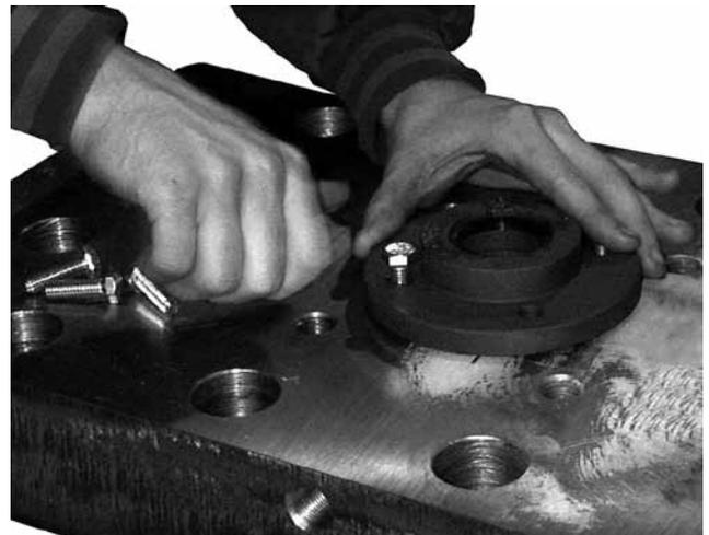
**5.7.22** Approaching from the top of the cupola, insert the new stem through the stem packing. Be careful not to damage the stem packing. Let the stem protrude from the bottom of the bonnet approximately the same amount as the old stem. Tighten the capscrews holding the bolted stem packing retainer to the cupola.
