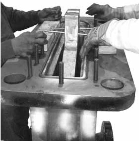
**5.3.24** Using proper equipment and lifting procedures, lift the entire top works assembly, including the cupola and bonnet, and place over the valve body.
