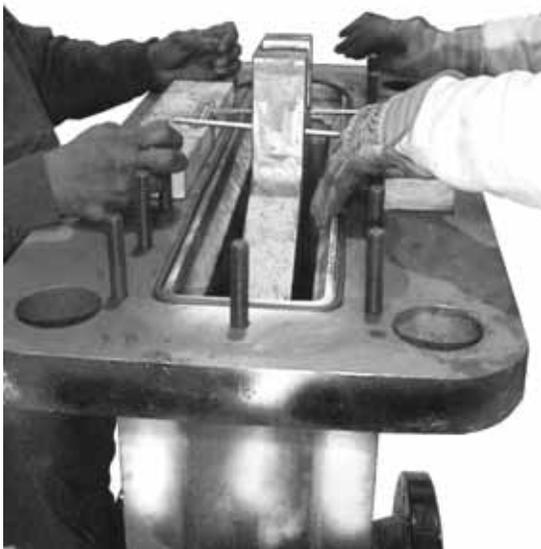
**5.7.28** Using proper equipment and lifting procedures, lift the entire top works assembly, including the bonnet, and place over the valve body.
