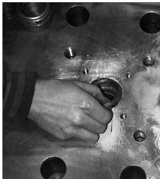
**5.4.14** Clean the stem packing area in the lower yoke flange. If the valve has a stem retainer, install it now and seat it in the counterbore located in the lower yoke flange. Reassemble the yoke to the cupola. **NOTE: Be careful not to damage the stem seal area of the stem when sliding the cupola over the stem.**
