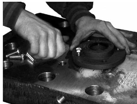
**5.5.21** Approaching from the top of the bonnet, insert the new stem through the stem packing. Be careful not to damage the stem packing. Let the stem protrude from the bottom of the bonnet approximately the same amount as the old stem. Tighten the capscrews holding the bolted stem packing retainer to bonnet.
