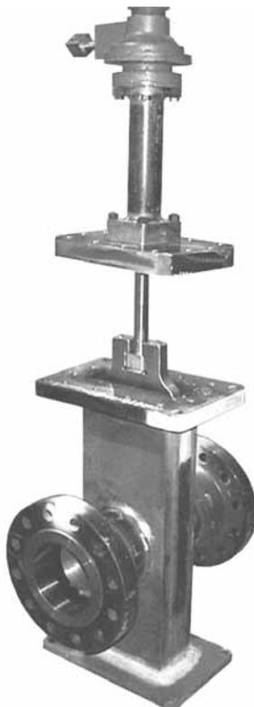
**5.6.7** Using proper equipment and lifting procedures, lift the entire top works assembly, bonnet, and gate high enough to clear the T-bar slot in the gate. Insert customer supplied drift pins in the holes provided in the bottom of the gate T-bar slot.
