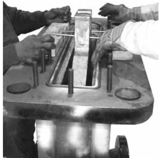
**6.1.17** Using proper equipment and lifting procedures, lift the entire top works assembly including the bonnet and slide the stem T-bar into the T-bar slot of the gate.
