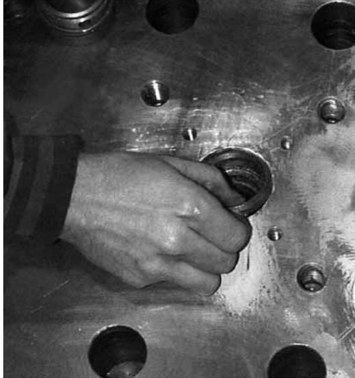
**5.6.18** Clean, inspect, and install the bolted stem packing retainer. The upper adapter ring of the stem packing should seat in the counterbore located in the bottom of the bolted stem packing retainer. Fasten to the bonnet using capscrews. **DO NOT** tighten capscrews at this time.
