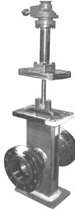
5.7.7 Using proper equipment and lifting procedures, lift the entire top works assembly, bonnet, cupola, and gate high enough to clear the T-bar slot in the gate. Insert customer supplied drift pins in the holes provided in the bottom of the gate T-bar slot.
