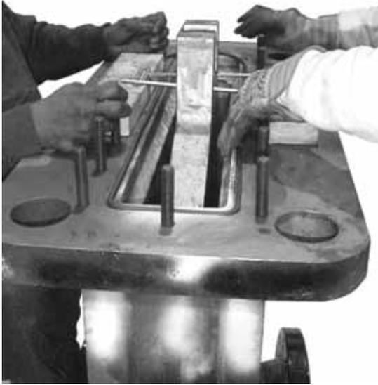
**5.8.25** Using proper equipment and lifting procedures, lift the entire top works assembly, including the bonnet, and place over the valve body.
