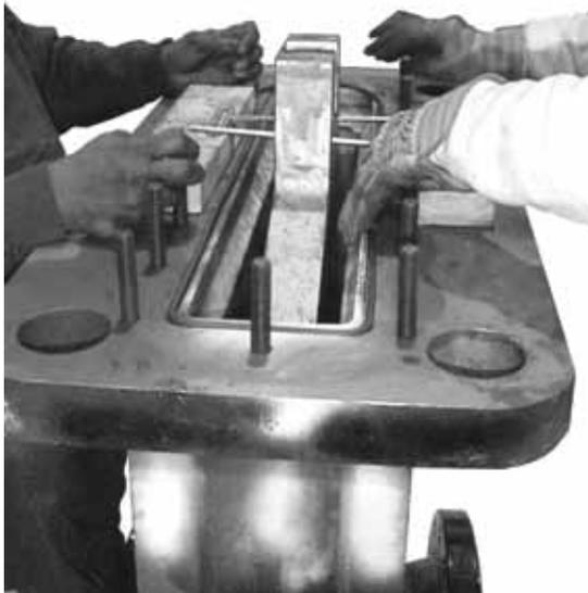
**5.5.28** Slide the T-bar into the T-bar slot on the top of the gate. Remove the drift pins if used and lower the complete topworks assembly and gate into the place with the bonnet resting on the body bolting flange.
