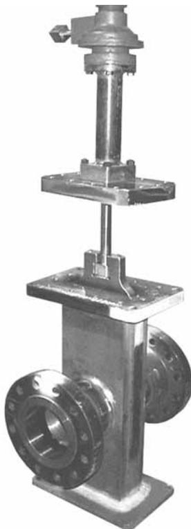
5.1.7 Using proper equipment and lifting procedures, lift the entire top works assembly, bonnet, and gate high enough to clear the T-bar slot in the gate neck. Insert customer supplied drift pins in the holes provided in the bottom of the gate neck T-bar slot.
