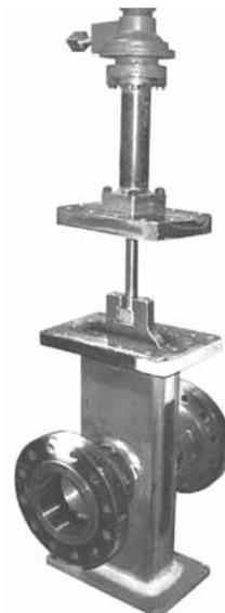
**5.2.7** Using proper equipment and lifting procedures, lift the entire top works assembly, bonnet, and gate high enough to clear the T-bar slot in the gate neck. Insert customer supplied drift pins in the holes provided in the bottom of the gate neck T-bar slot.
