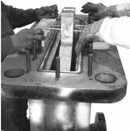
**5.4.20** Using proper equipment and lifting procedures, lift the entire top works assembly, including the cupola and bonnet, and place over the valve body.
