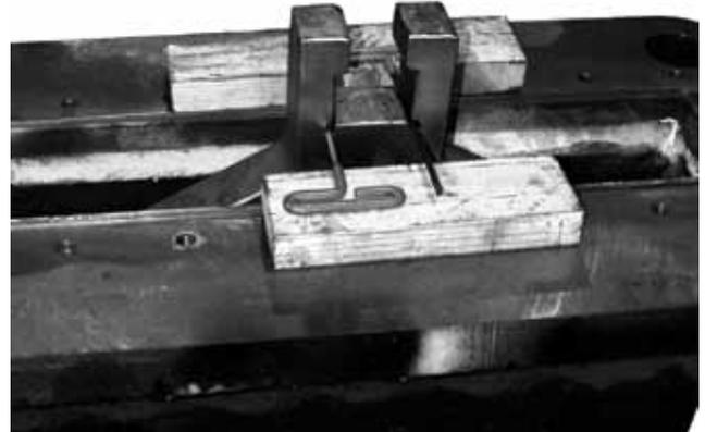
**5.5.8** Slide the stem T-bar out of the T-bar slot in the gate neck. This will disengage the top works assembly from the gate allowing its removal. Remove the bonnet O-ring.
