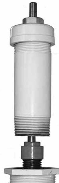
5.3.6 Remove bonnet nuts. Studs may also be removed, if desired, to allow more work clearance.
