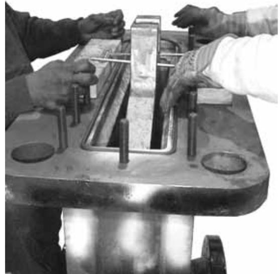
**5.2.17** Using proper equipment and lifting procedures, lift the entire top works assembly, including the bonnet, and place over the valve body.
