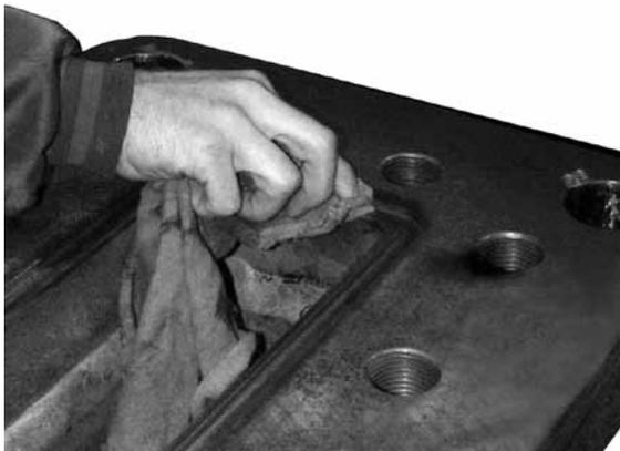
**5.2.13** Clean the stem packing area in the lower yoke flange. If the valve has a stem bushing, install it now and seat it in the counterbore located in the lower yoke flange. Reassemble the yoke to the bonnet. **DO NOT TIGHTEN BOLTS AT THIS TIME.**
