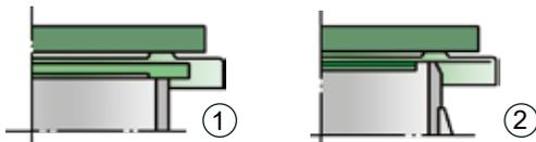
This “full lift type” technology allows the valve to be set at just 10% below the maximum allowable working pressure of the tank and still safely vent the required mass flow.
