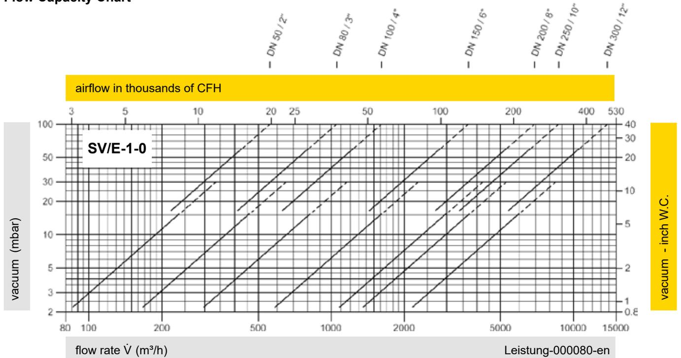
The flow capacity charts have been determined with a calibrated and TÜV certified flow capacity test rig. Volume flow  $\dot{V}$  in (m<sup>3</sup>/h) and CFH refer to the standard reference conditions of air in ISO 6358 (20°C, 1bar). For conversion to other densities and temperatures, refer to Sec. 1: "Technical Fundamentals."
